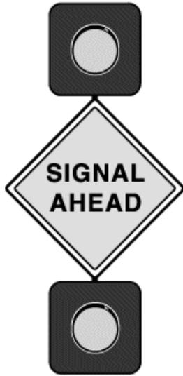
Flashing beacons (sometimes called flashers or flashing lights) are frequently requested in the belief that they will slow down traffic. However, the real purpose of flashers is to attract attention to unexpected hazards in the roadway.
