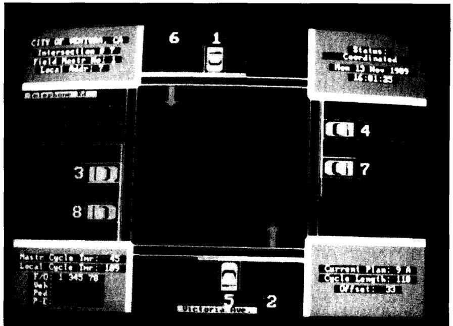
Figure 3. Real time intersection display.
