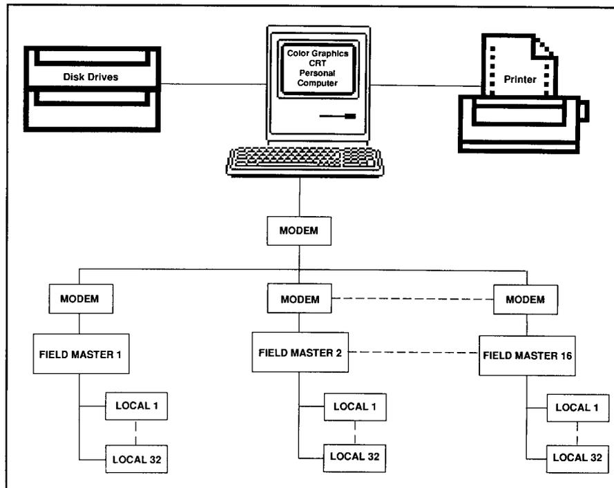
Figure 1. Traffic signal control and surveillance system.
