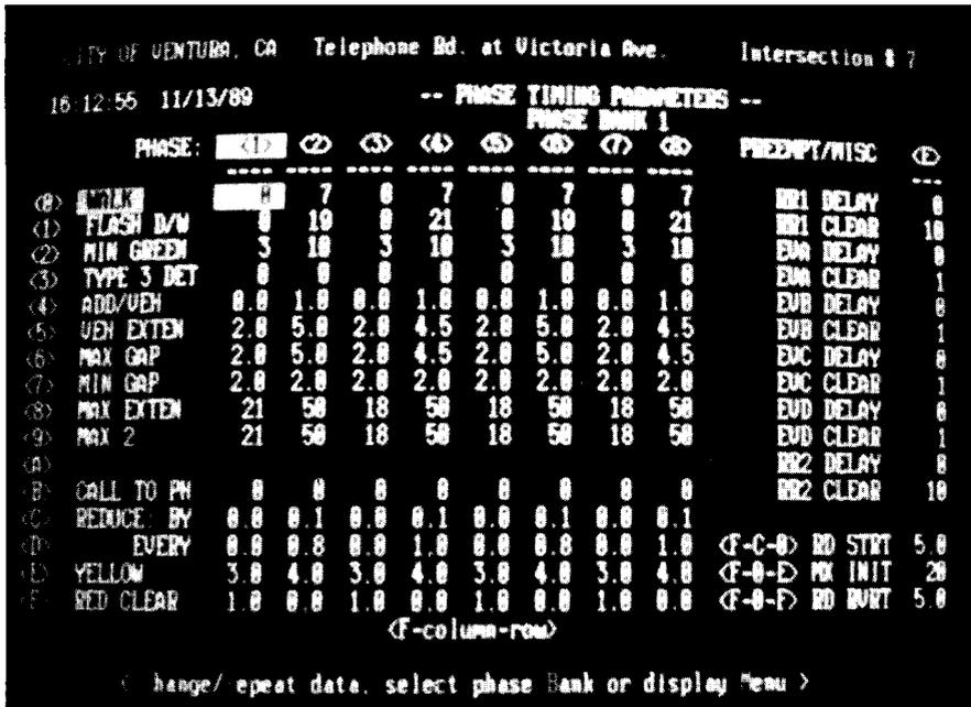
Figure 4. Signal timing data display.
