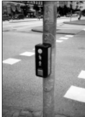
**Figure 5. Pushbutton with tactile map on the side includes sound generator, tactile map, LED light and vibrating hardware for accessibility.**
